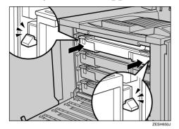
When there is a white line showing at the stoppers, reinsert the unit by following step **7**.
