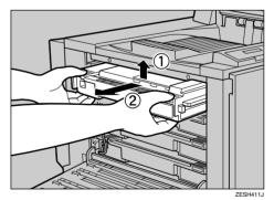
The illustration shows how to remove the black development unit. The procedure is the same for all four colors.
