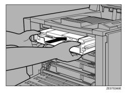
Confirm the label for the color, and then confirm that the unit is securely fit in the stoppers.
