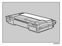
Set the new development unit by aligning the guides, pushing towards direction (1), and then inserting slowly until it stops (2).
