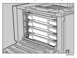
Detach the connectors from the development units from the top to the bottom by pressing the sides of the connectors.
