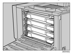
Detach the connectors from the development units from the top to the bottom by pressing the sides of the connectors.
